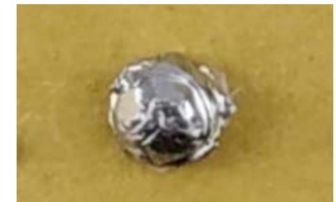
Palladium extracted using metal adsorbent
