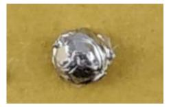
Palladium extracted using metal adsorbent
