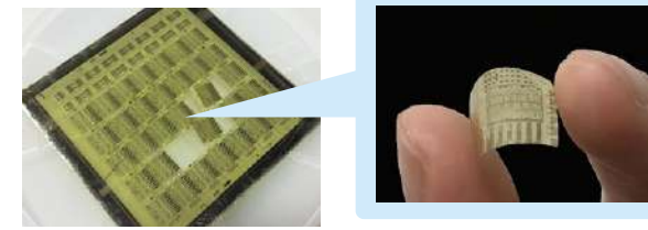
Flexible organic semiconductor made with a film-coating technology developed solely by PI-CRYSTAL
