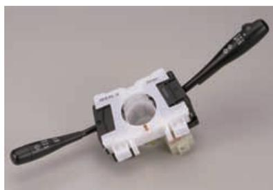
Polyacetal are used in Parts of Combination Switches.
