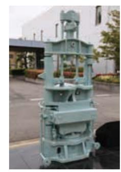
Celluloid manufacturing test equipment (press machine)
