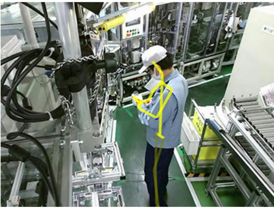
An example of the sensing system in action and how the image analysis system monitors the action of frontline operators
