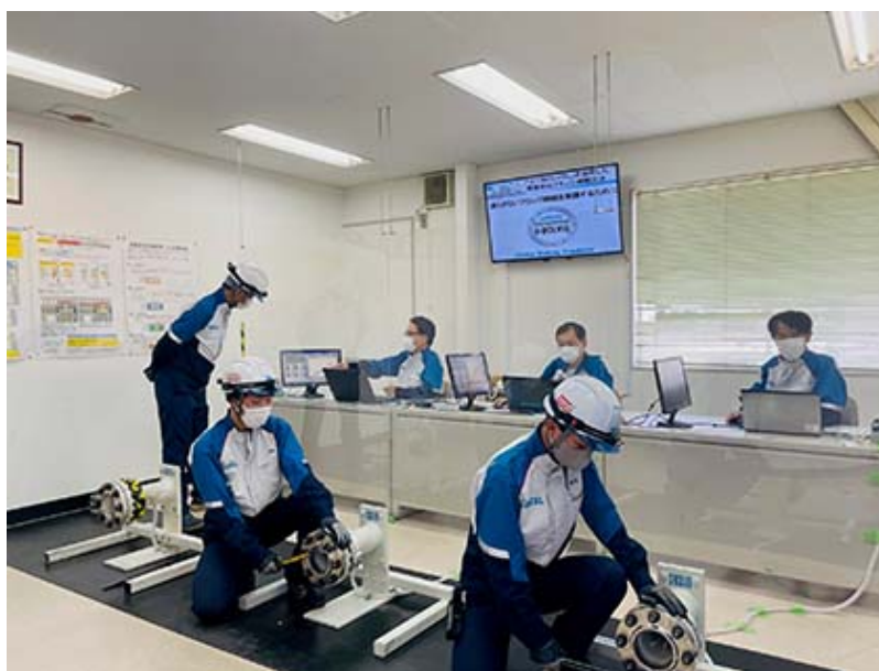
(Photo 2) Simulator-based scientific training for flange tightening
