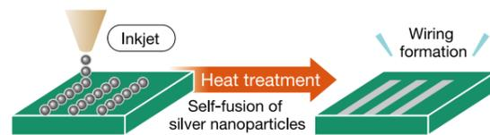
After printing the circuit, silver nanoparticles are heat treated to form the wiring. Compared to other brands, Picosil<sup>®</sup> can be treated at a lower temperature range of 120°C to 150°C so that circuits can also be formed on PET resins. Various types of printing methods, such as inkjet, screen, gravure, and offset printing, can be used for the application, and with the inkjet printing method, circuits can be formed by drop-on-demand printing.
