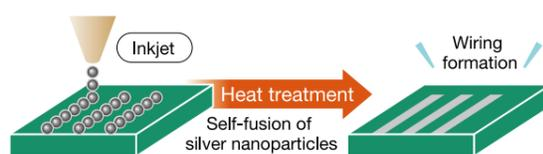
After printing the circuit, silver nanoparticles are heat treated to form the wiring. Compared to other brands, Picosil<sup>®</sup> can be treated at a lower temperature range of 120°C to 150°C so that circuits can also be formed on PET resins. Various types of printing methods, such as inkjet, screen, gravure, and offset printing, can be used for the application, and with the inkjet printing method, circuits can be formed by drop-on-demand printing.
