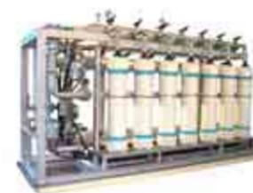
Water purification system using separation membranes
